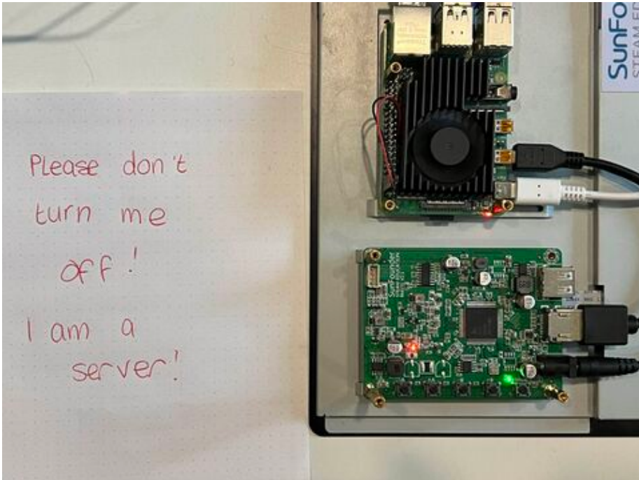
Figure 8: Photograph from Transmediale Content/Form Workshop 2024. It depicts the Raspberry Pi used to host the publishing infrastructure of a web2print publication created during the workshop.
